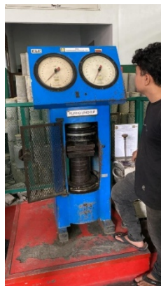
Gambar 3 Alat Uji Kuat Tekan (Compression Testing Machine)
