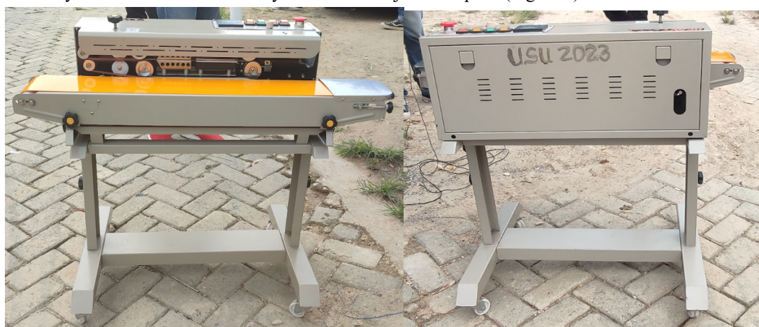
Figure2. Continuous band sealer machine provided to Partners.
