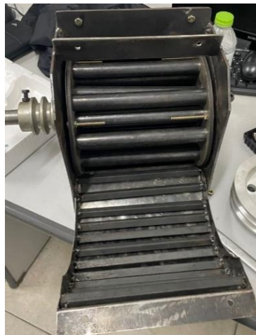
Gambar 8. Perakitan Ripple Plate
