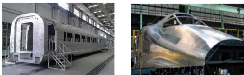
Gambar 1. Aplikasi *aluminum alloy* pada *car-body shinkansen 300 series high speed train* [3]
