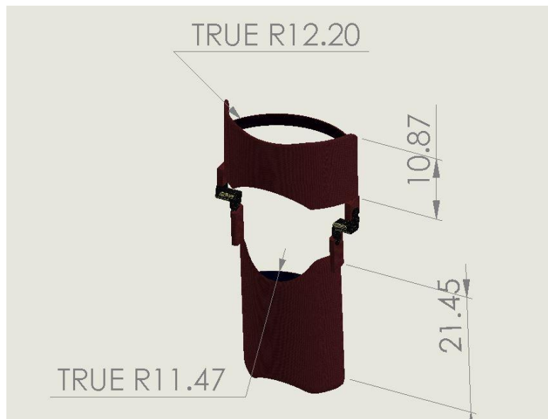
Gambar 1. Hasil Rancangan Akhir Knee and Leg Brace
