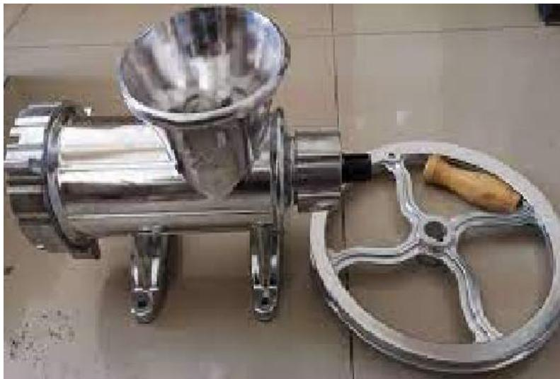
Gambar 2. Mesin Giling Daging Manual
